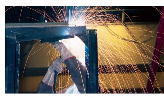
Close to a half million welders are affected by this standard, although chromates can also be present in various industries involving photographic pigments, dyes, surface coatings, paints, inks, plastics, thermal cutting, chrome plating, and stainless steel fabrication.
